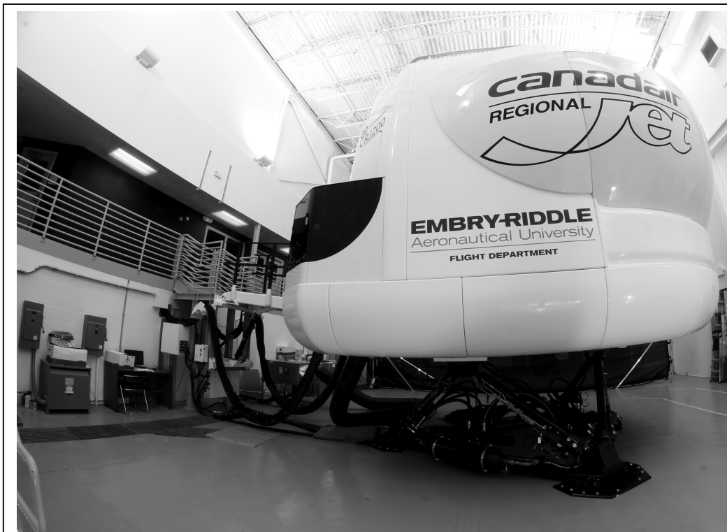
Figure 1. A CRJ 200 full-flight simulator. This is typical of those required by the new FAA rule for first officer qualification.
