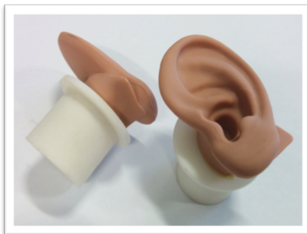
Figure 4: The 3D printed ear simulation.
