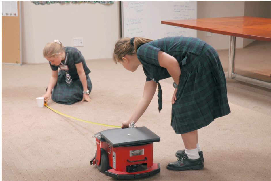
Figure 2: Picture of one team performing a translational error experiment.
