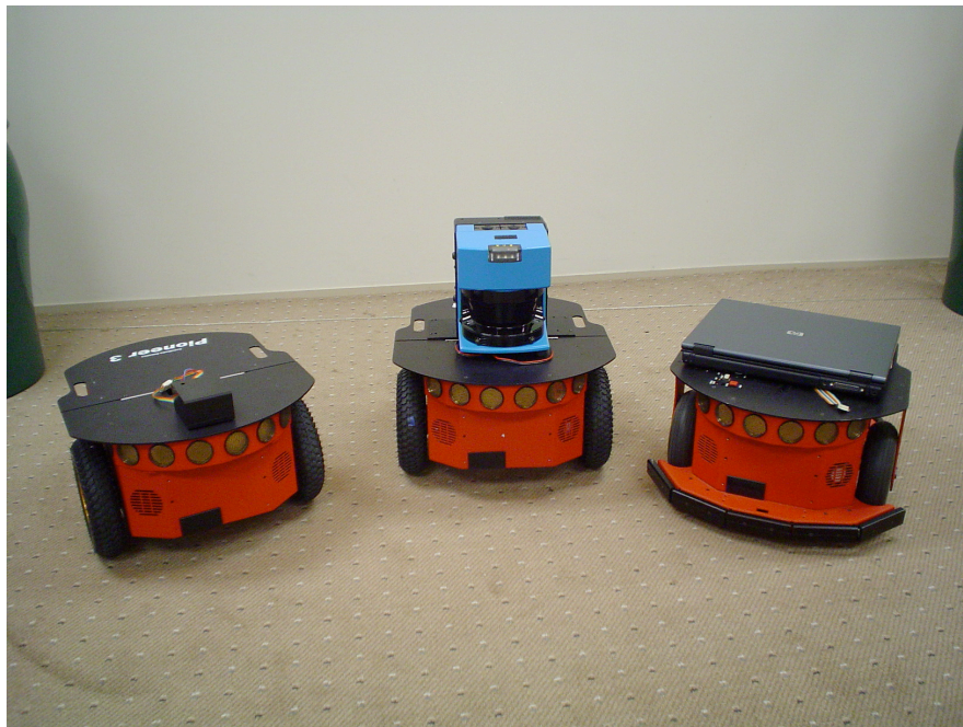
Figure 1: The three Pioneer robots used for the course. Each is equipped with eight sonar sensors, the one in the middle has an additional laser range finder.
